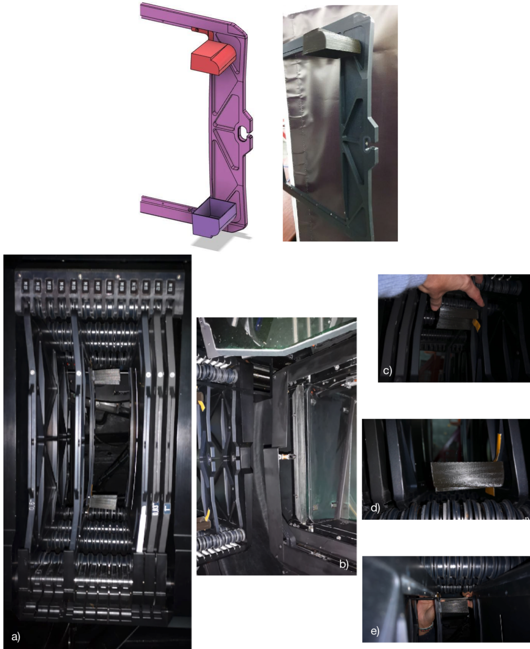
Figure 18. Top: 3D printed dummies built for the in situ testing of the MAAT envelope on OSIRIS (Credit: GTC). Bottom: In situ testing of the dummy of the MAAT module on OSIRIS: a) MAAT envelope dummy placed in the Loader mask, b) Baffle to redesign in order to accommodate the subsystem mask frame plus MAAT envelope, c) Width of the MAAT envelope, d) Free space between the rollers and the lower part of the MAAT envelope (orientation rotB = 80^\circ ), and e) Free space between the upper part of the MAAT envelope and the masks edge protection (orientation rotB = 80^\circ ). All these pictures have been taken with orientation of rotB = 80^\circ . (Credit: GTC).
