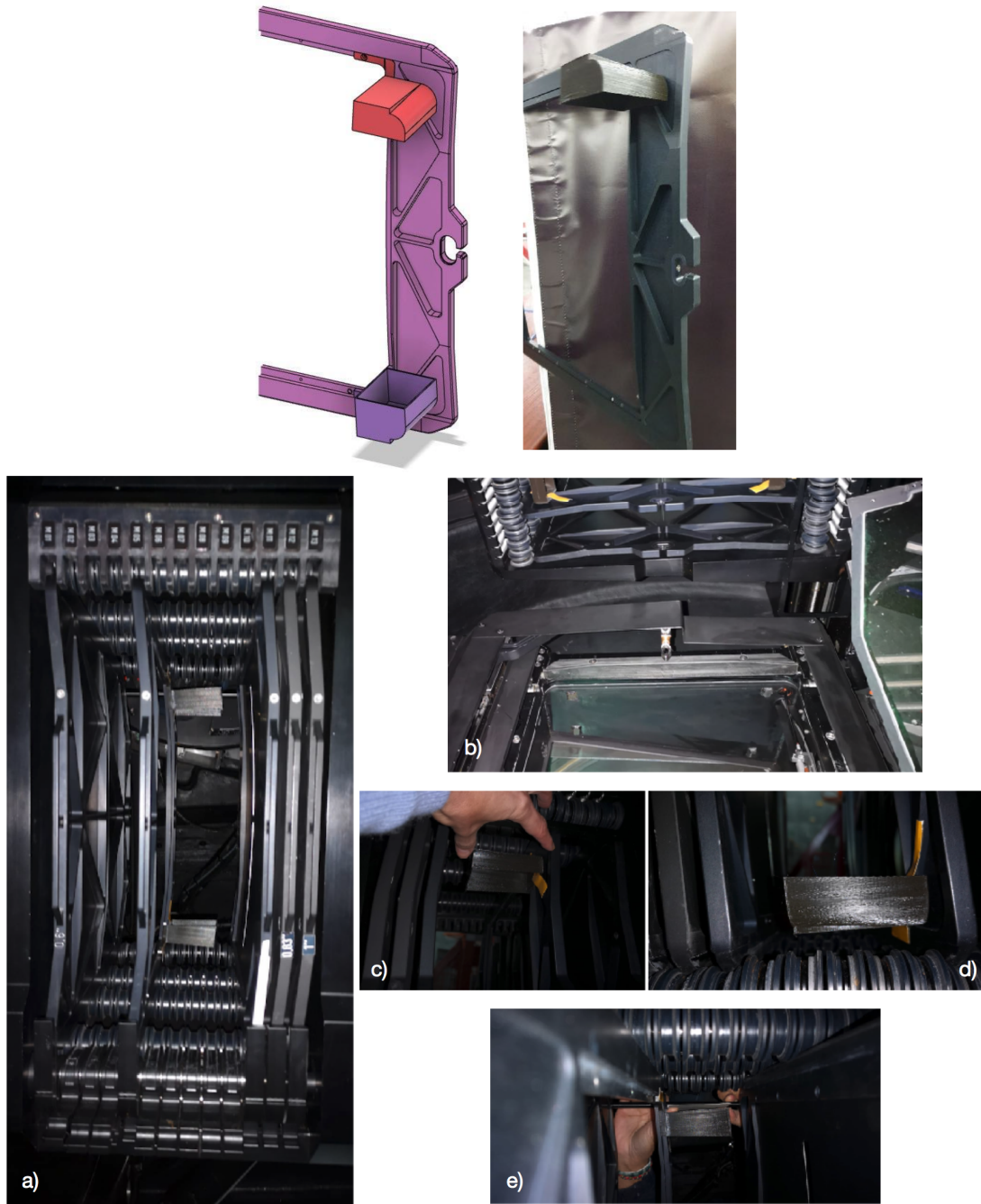
Figure 19. Top: 3D printed dummies built for the in situ testing of the MAAT envelope on OSIRIS (Credit: GTC). Bottom: In situ testing of the dummy of the MAAT module on OSIRIS: a) ..., b) ..., c) ..., d) ..., and e) ... (Credit: GTC).
