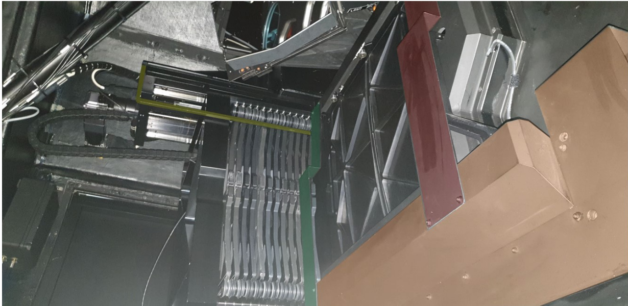
Figure 19. Picture of the OSIRIS Cartridge and focal plane assembly as built. In green, red, and brown are highlighted different metal pieces which are described in the text (Credit: GTC).
