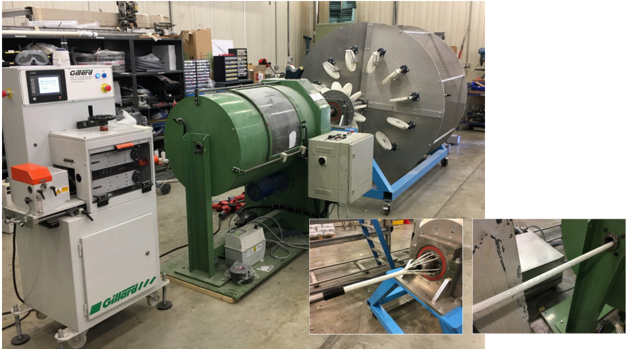
Anticlockwise from top right: More pictures of the strander and the production line, finished cable core, putting the cable core into conduit.
